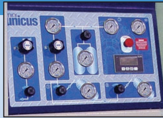
Cascade Fill Control Panel with Air Flow Schematic
